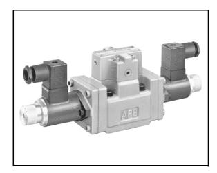
This directional and flow control valve enables remote control of the direction and flow of hydraulic fluid by controlling the solenoid input current. The flow can be controlled steplessly in proportion to the current value.
