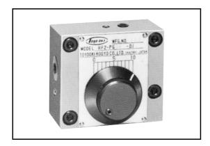
This valve controls flow by changing the cross-sectional area through which fluid flows. Since it incorporates a pressure compensation mechanism, the flow is kept constant even if the pressure varies at the IN and/or OUT port.
