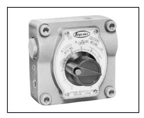
This valve controls flow by changing the cross-sectional area through which fluid flows. Since it incorporates pressure compensation mechanism and temperature compensation mechanism, the flow is kept constant regardless of the pressure variation at the IN and/or OUT port and the viscosity variation due to temperature change.
