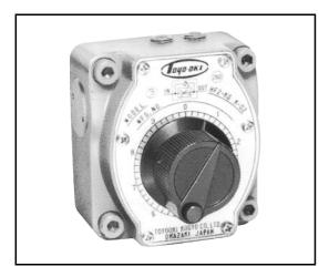
This valve controls flow by changing the cross-sectional area through which fluid flows. Since it incorporates pressure compensation mechanism and temperature compensation mechanism, the flow is kept constant regardless of the pressure variation at the IN and/or OUT port and the viscosity variation due to temperature change.
